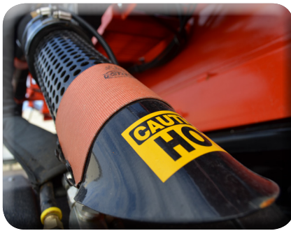
Vent-Flo nozzle with optional heater
